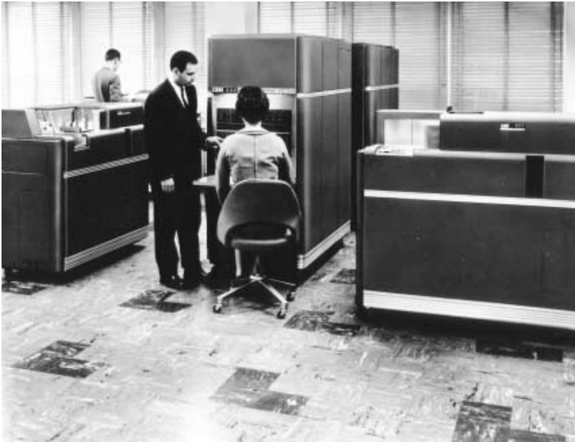
A typical IBM 650 Data Processing System, with card reader and printer, 1953.
